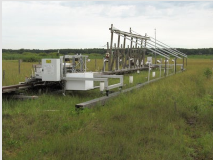
Photo 5. A technically advanced automatic greenhouse gas balance measurement station and for experiments with changing rainfall and temperature, on the Rzezińskie mire in the Notecka Forest in Greater Poland. Photo by J. and P. Pawlaczyk.
